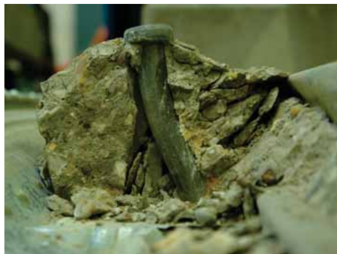
Figure 3: Failed stud in transverse trapezoidal decking (courtesy University of Luxembourg)
