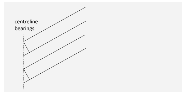
Figure 4 Skew deck with bracing square to beams
