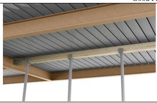
Props normally consist of lengths of timber and/or steel plates supported by adjustable length steel tubes (acrow props). The minimum bearing length of the timber and/or plates depends upon the thickness of the slab, the span length and the deck rib geometry.
