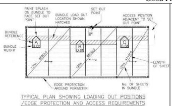
The Decking/Studwelding Contractor will provide loading out drawings indicating the required positions for individual bundles, the direction of span and orientation of the bundle.
