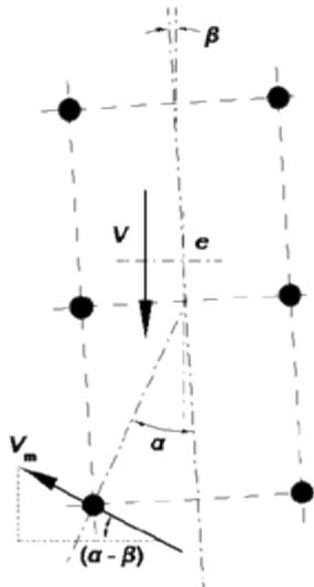
For the stud shown, the horizontal component =  $V_m \cos (\alpha - \beta)$ ; the vertical component =  $V_m \sin (\alpha - \beta)$
