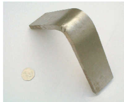
Bend test (note opening of root defect)
