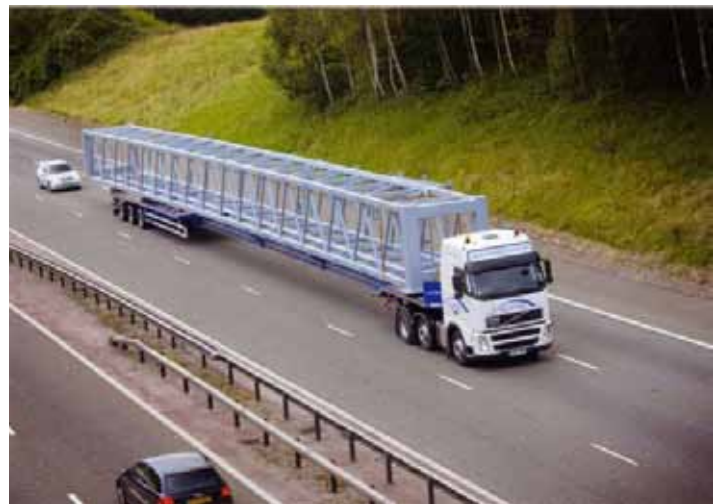
On its way: A prefabricated gantry section is transported to site
