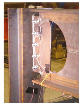
Figure 4 - Buckling of the half infill plate due to the transfer of shear from the top Tee
