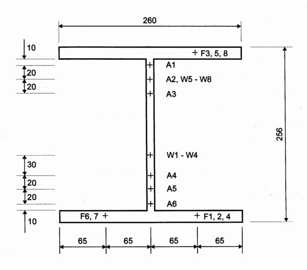
FIG. 5 THERMOCOUPLE POSITIONS IN THE STEELWORK - (D0229C06)
