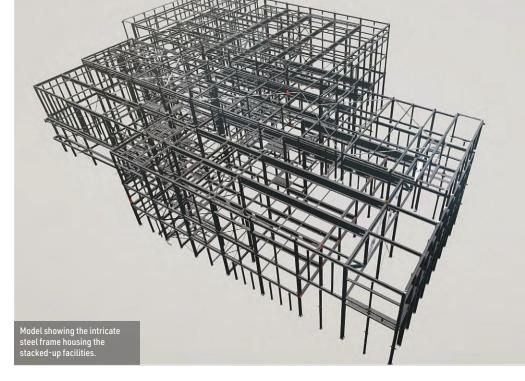
by a series of 14m-long  $\times$  1m-deep beams that support the column line for first-floor fitness suite.
