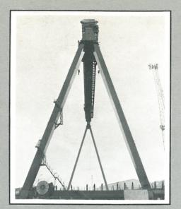
The crane is designed for transporting large prefabricated parts of ships, up to 225 tons each, and holding them accurately in position while they are welded to the main structure.
