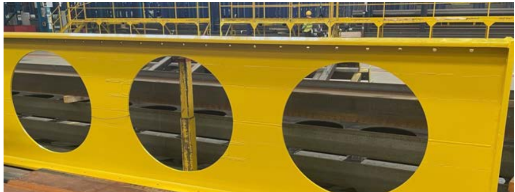
Refabricated 1300 mm deep cellular beam
