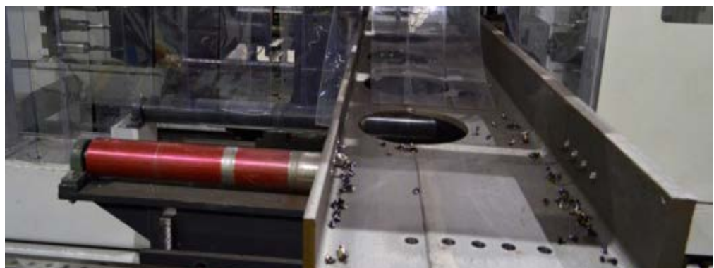
Figure 7.6 Asymmetric cellular beam fabricated from rolled sections
