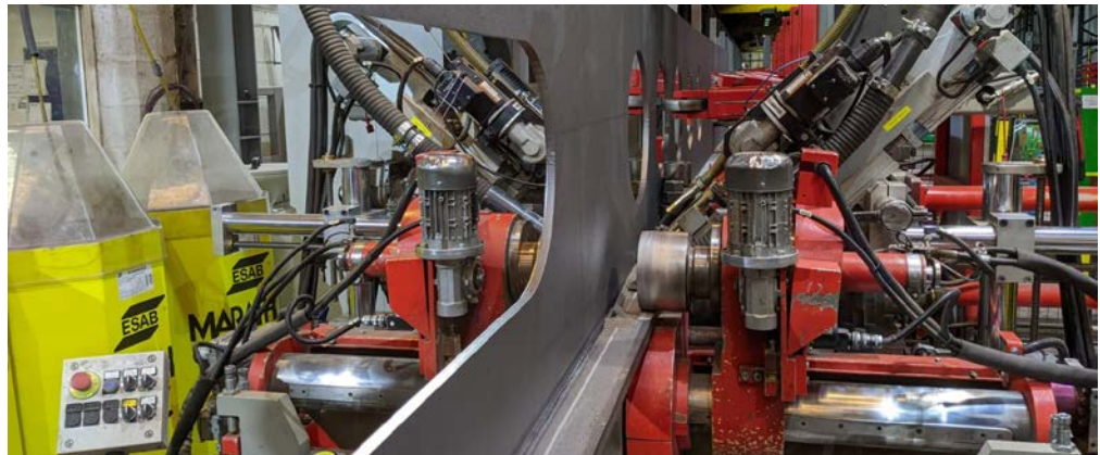
Figure 7.5 Asymmetric section fabricated from plate
