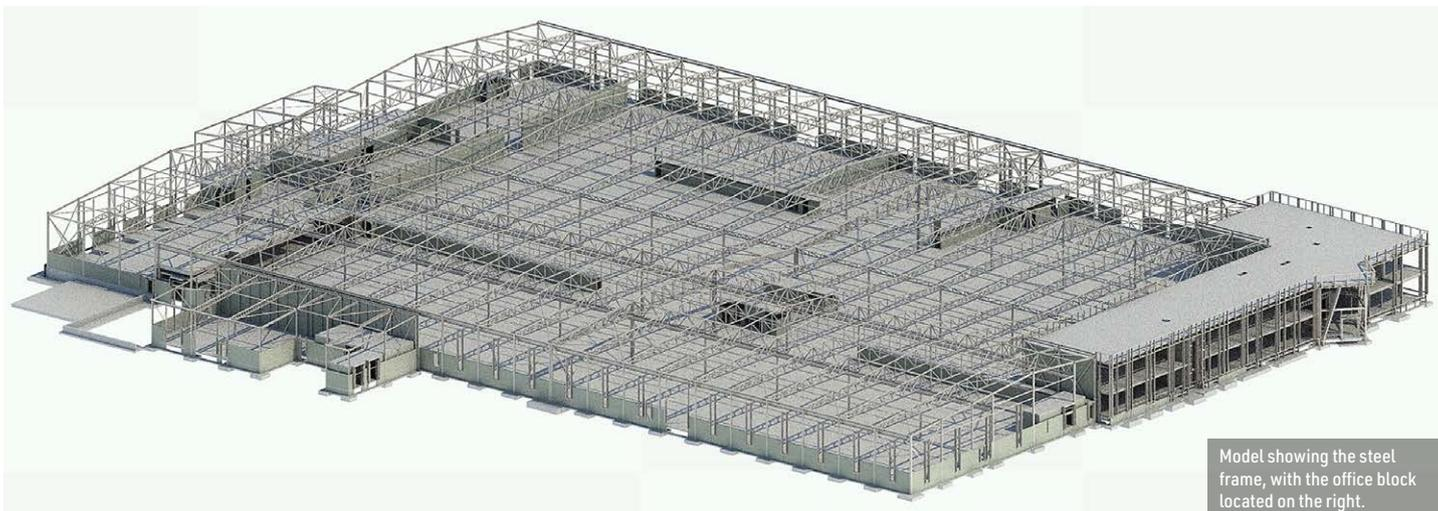
Model showing the steel frame, with the office block located on the right.
