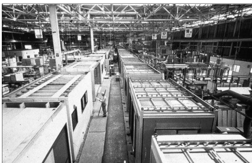
Figure 4.1 Production of Japanese modular units
