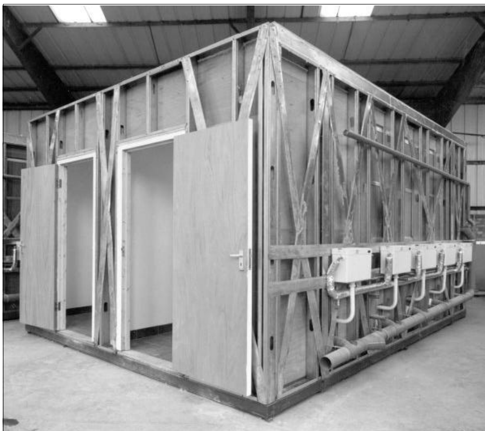
Figure 2.2 Toilet pods for use in commercial buildings
