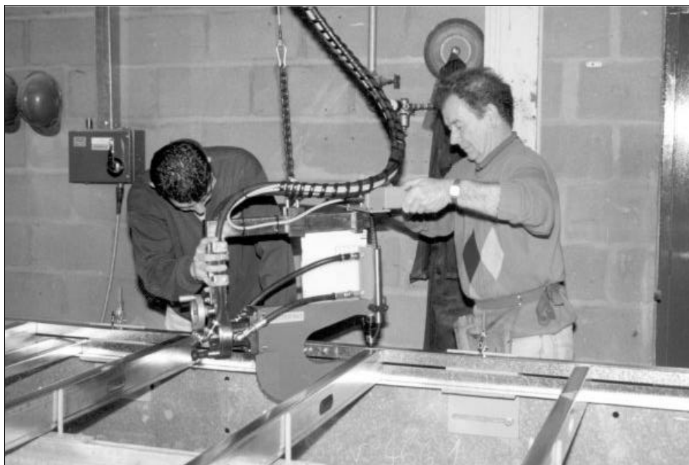
Figure 6.1 Connections using self piercing rivets
