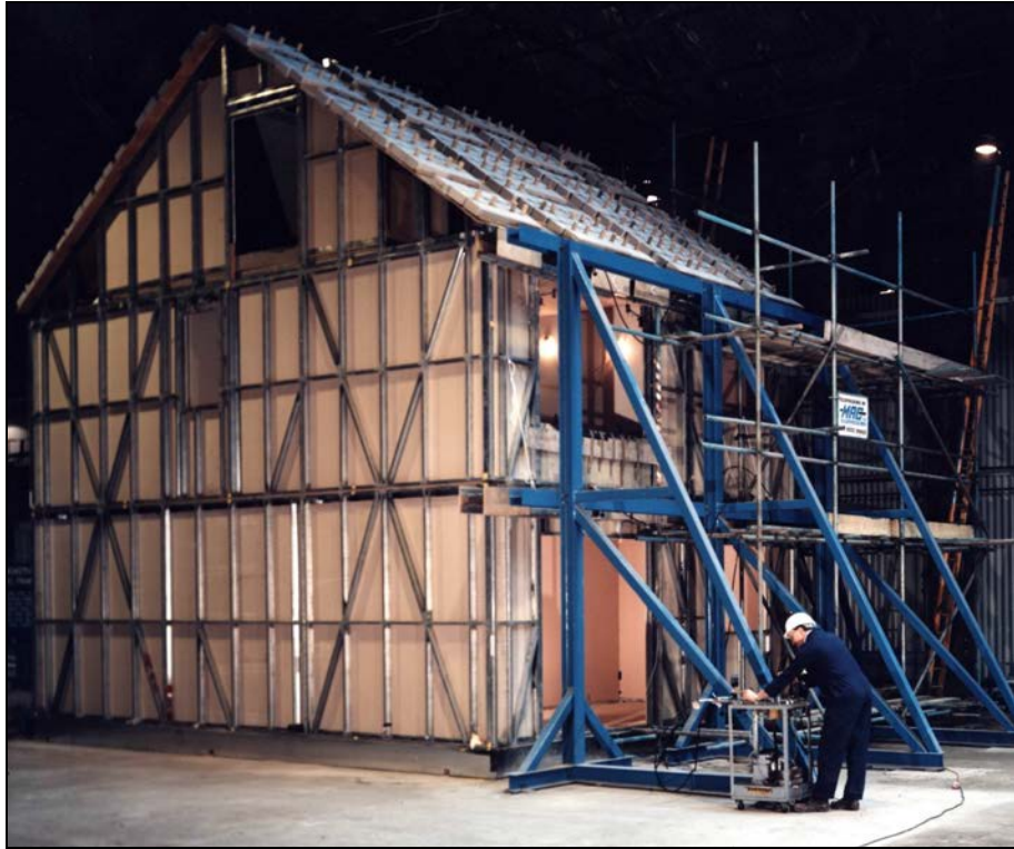
Figure 4.12 Light steel framing with open roof system under test
