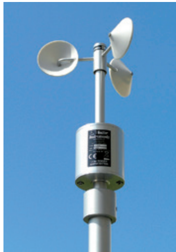
Figure 2.1 Cup Anemometer by Vector Instruments Courtesy of Windspeed Ltd.
