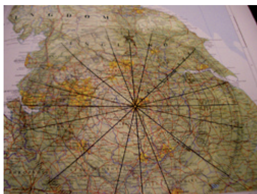
Figure 5.6 SCI wind protractor centred at Sheffield on 1:1000 000 map The Times Atlas of the World (www.timesatlas.com) © Collins Bartholomew
