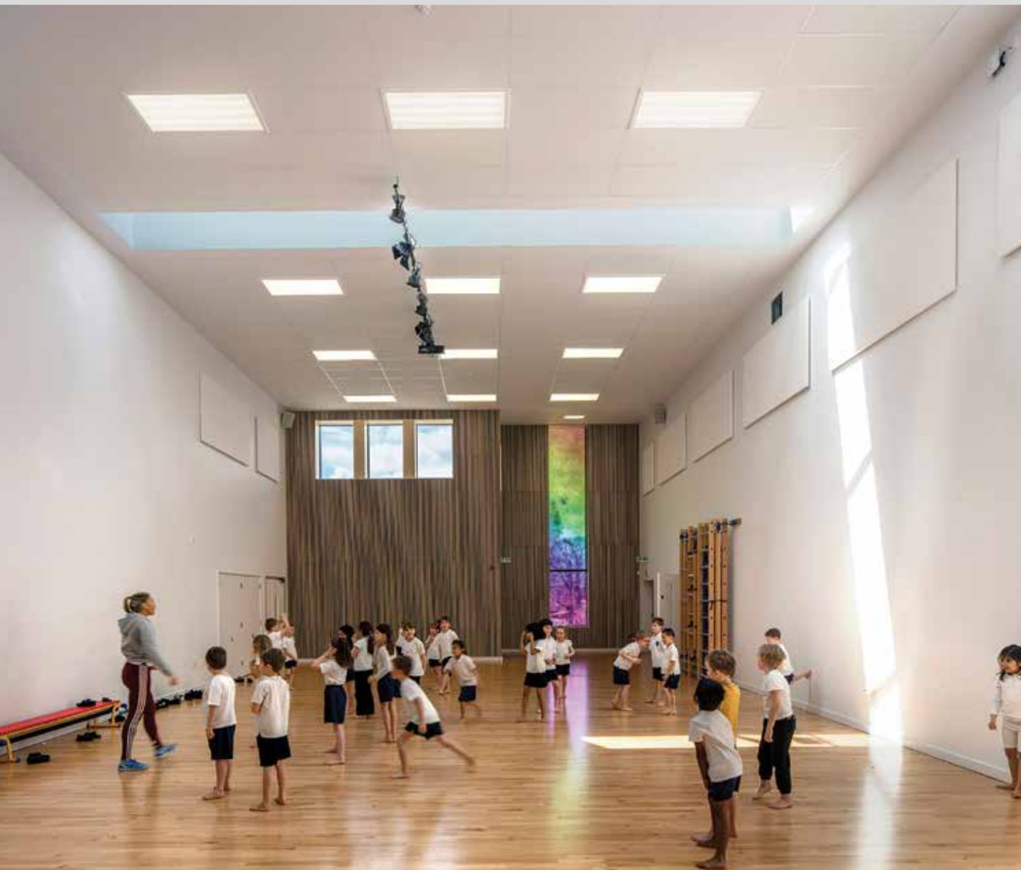
Left A transfer structure enables a column-free sports hall within the two-storey communal component of the radial school.
