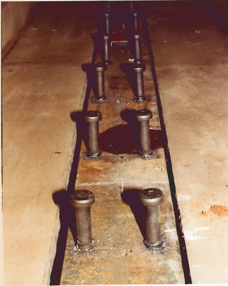
SHEAR STUDS WELDED ONTO THE TOP FLANGE OF THE TEST BEAM. FIGURE 2.
