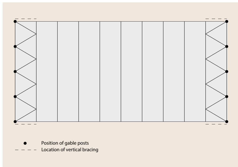
Figure 8.8 Plan view showing both end bays braced
