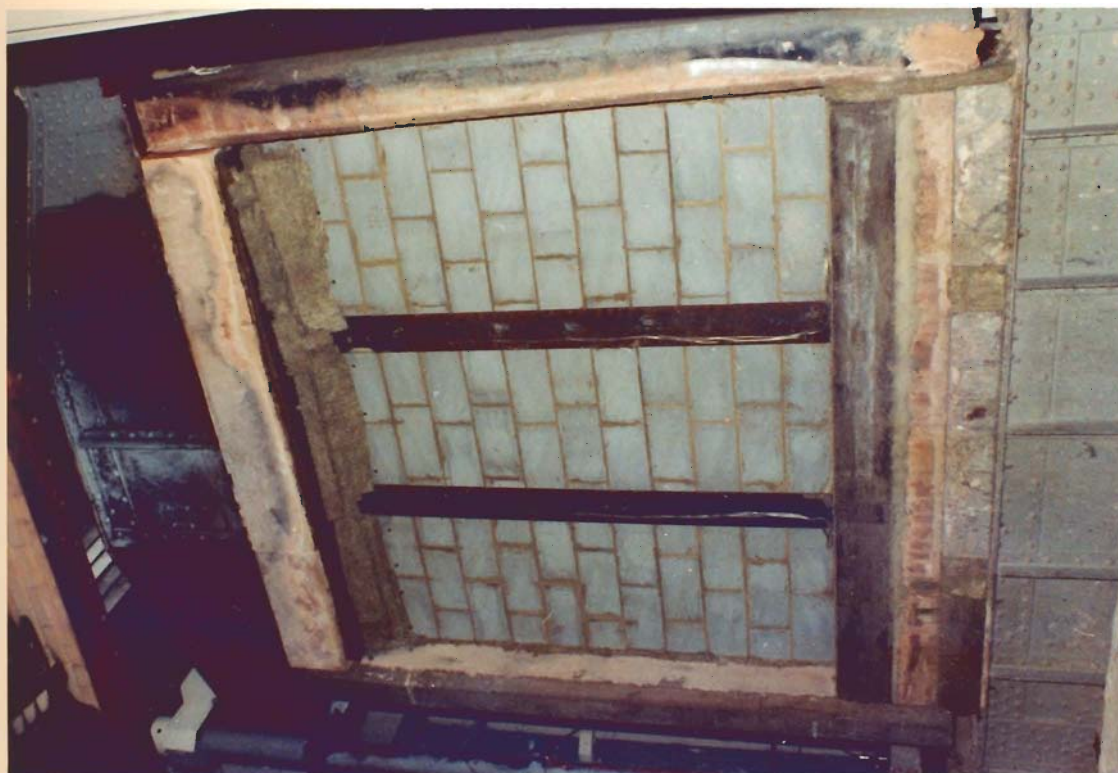
FINAL CONSTRUCTION POSITIONED IN FURNACE SHOWING THE EXPOSED AND UNEXPOSED SIDES
