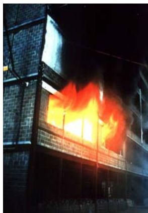
(a) Fire (Cardington test)
