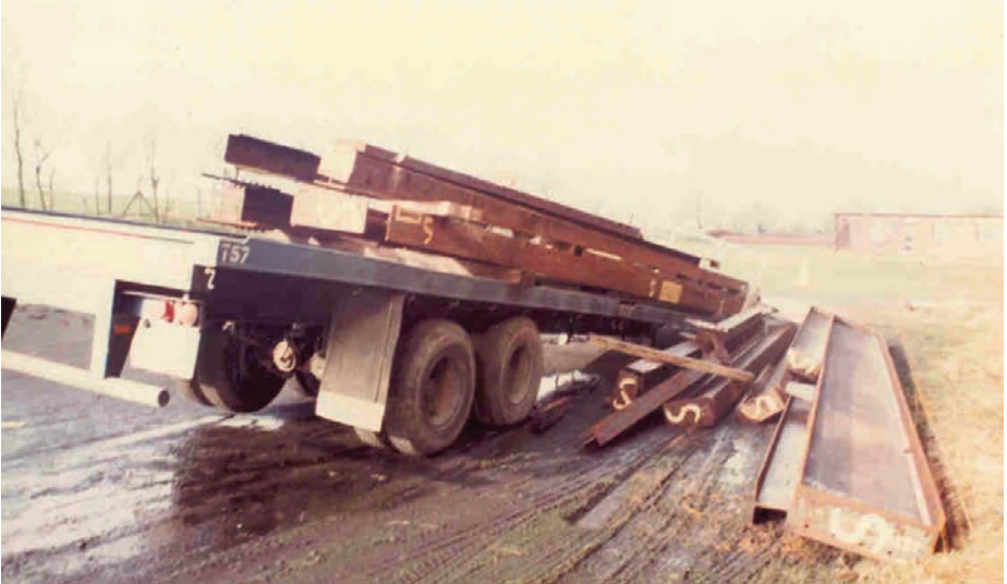
How poor ground conditions can affect loaded trailers
