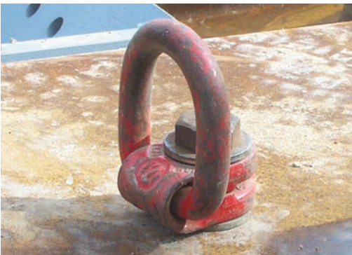
Lifting aid bolted to steelwork
