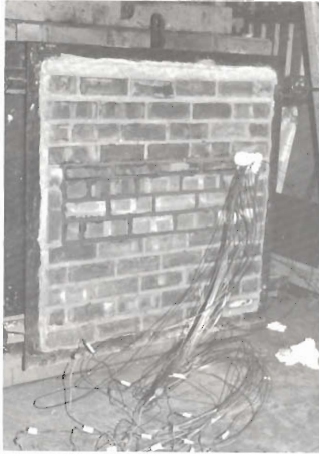
THE 1 m CUBE FURNACE AT WARRINGTON RESEARCH CENTRE SHOWING THE UNEXPOSED SURFACE OF A PERIMETER BEAM SET IN THE WALL FIG. 24(a)
