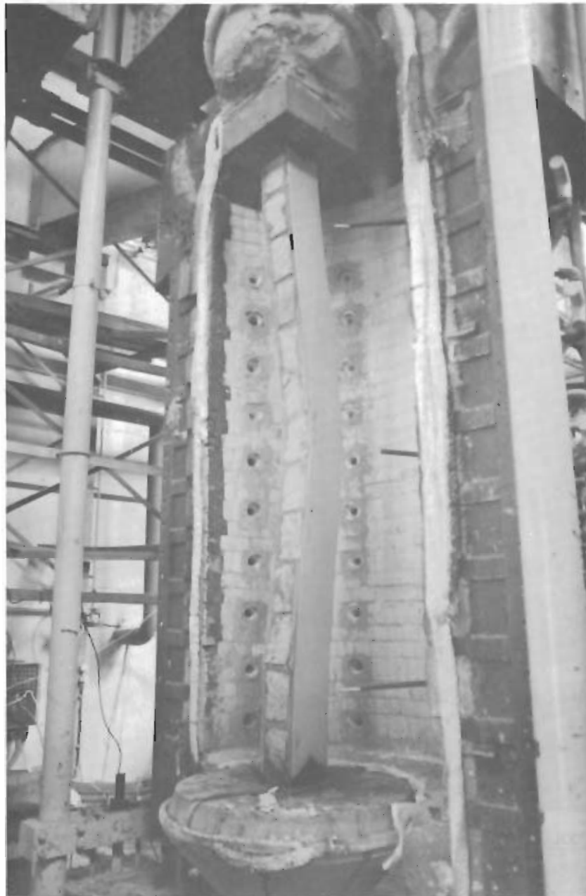
A STEEL COLUMN WITH A BLOCKED IN WEB FOLLOWING A FIRE TEST FIG. 14(b)
