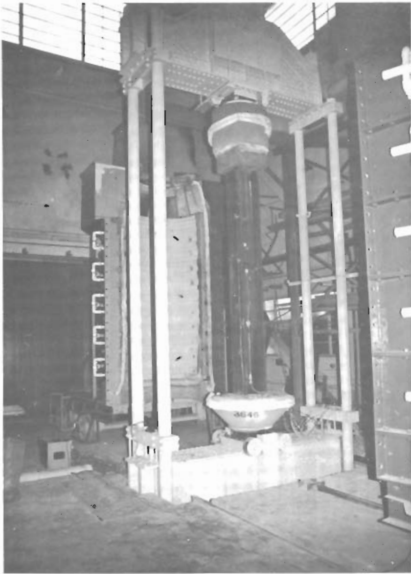
THE COLUMN FURNACE FIRE TEST FACILITY AT FIRTO, BOREHAMWOOD FIG. 14 (a)
