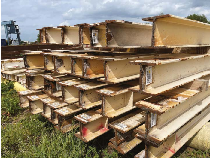
Figure 1: Recovered steel members (courtesy Cleveland Steel & Tubes Ltd)
