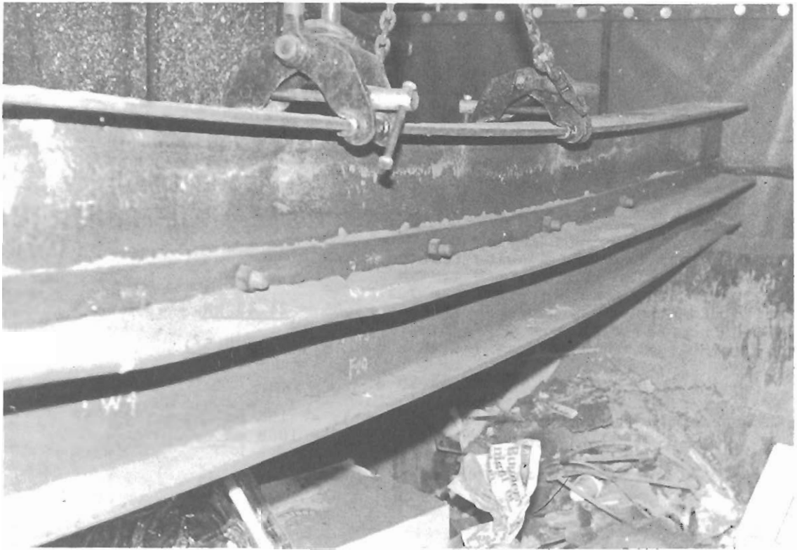
WAVEY PATTERN FORMED ALONG THE SHELF ANGLE DURING THE TEST
