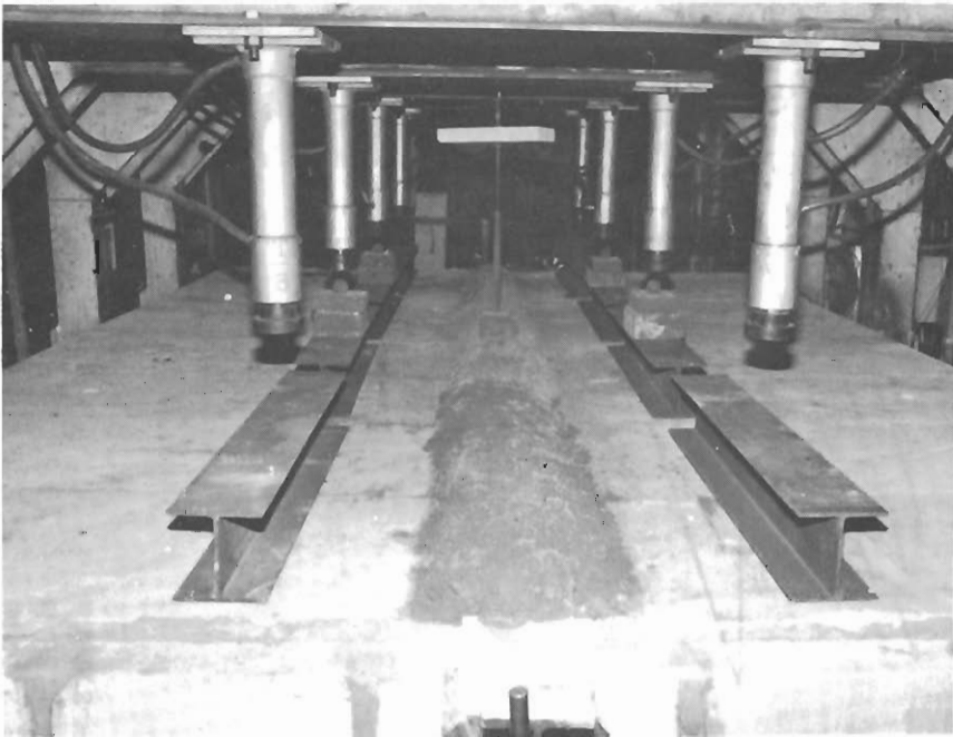
TEST ARRANGEMENT WITH 150 mm THICK FLOOR SLABS PRIOR TO TESTING FIG. 7
