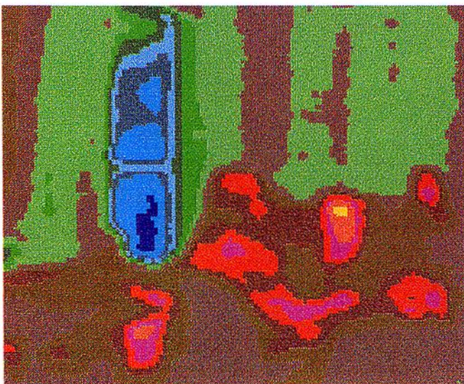
THERMAL IMAGE INDICATING SOURCES OF AMBIENT HEAT GAINS IN A TYPICAL OFFICE ENVIRONMENT
