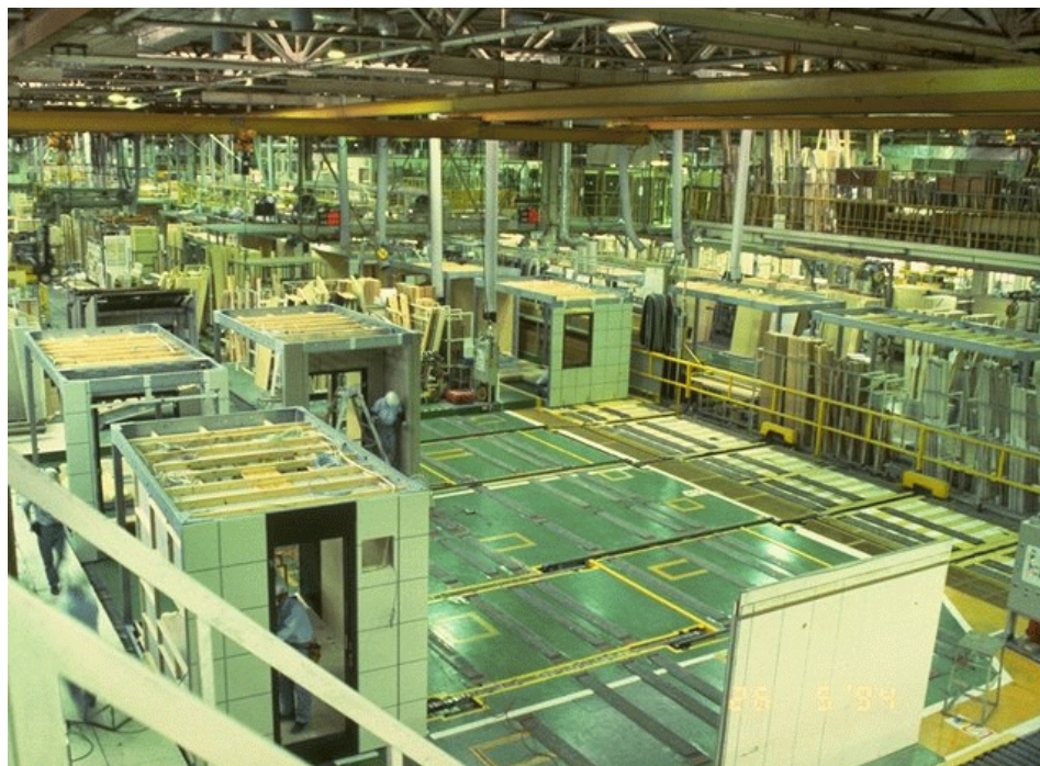
Figure 1.6 Modular units are produced in a controlled environment to high quality
