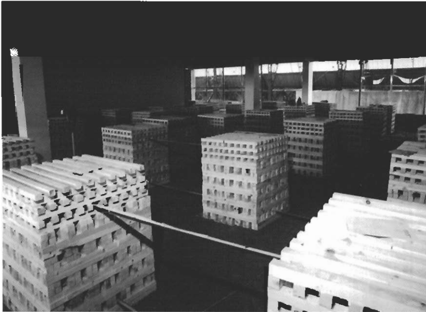
Figure 6.34 Timber cribs within the compartment
