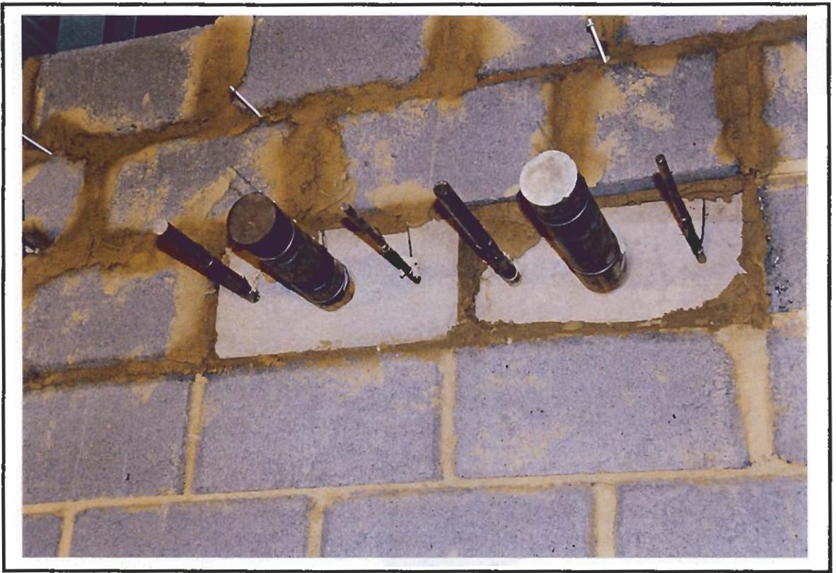
Fig. 10 Steel Bars Set in 100 and 190 mm Thick Concrete Blocks (Compartment Interior View, 190 mm Block on Left)
