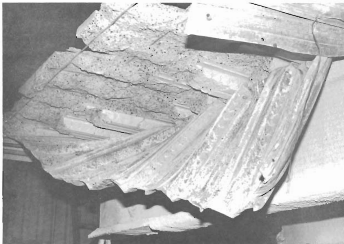
LIGHTWEIGHT CONCRETE ON CF46 DECK AFTER 105 min
